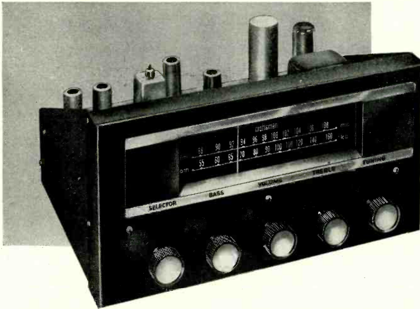
Fig. 1—Radio Craftsmen type 800 tuner.
